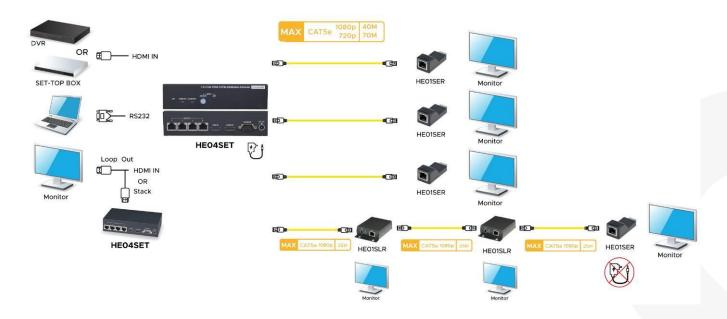
Stack to another HE04SET through HDMI loop out port to get configuration of 1 in 8 out.
